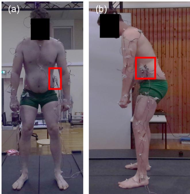
Fig. 3. Subject wearing the synchronized markers in a) frontal view and b) side view. Red Rectangle: Power distributor. Excess wire is spun in a loop and taped to the skin. For privacy reasons, the image is anonymized.
