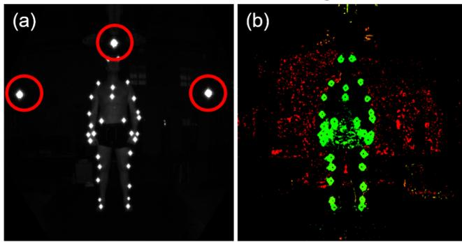
Fig. 6. Impact of active noise generated on image quality. a) Infrared image. Red circle: Vicon camera. b) Almost completely corrupted corresponding depth image
