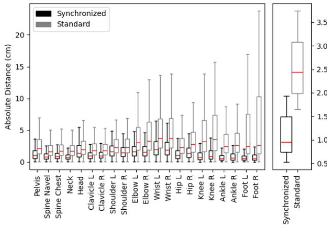
Fig. 9. Mean absolute error of every zero-mean shifted joint in every recording for synchronized and standard markers. Right: Boxplot of all medians. Outliers were removed to improve visibility.
