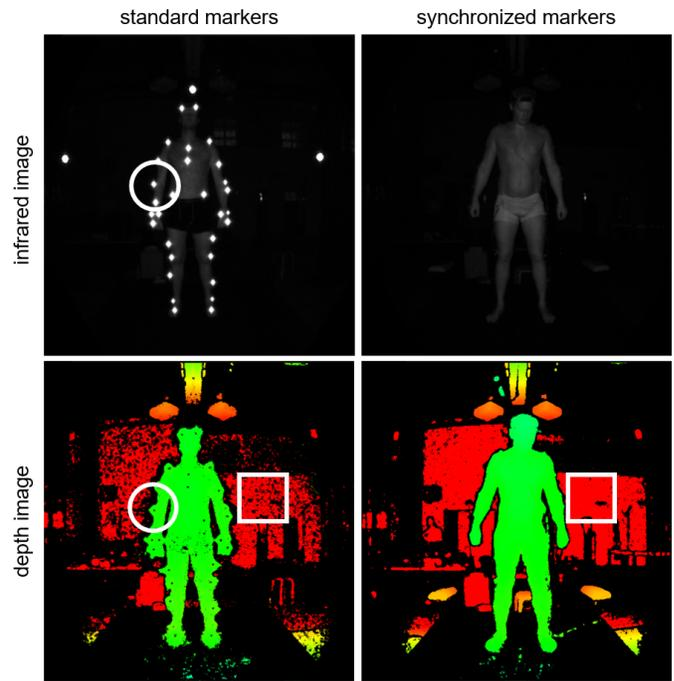
Fig. 4. Comparison of infrared (upper row) and depth image (lower row) of the Kinect when using the standard markers (left column) or the novel synchronized markers (right column). White circle: highlighting of a marker. White square: highlighting of the active noise.
