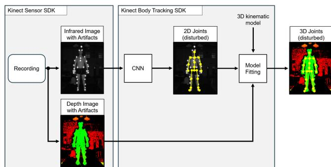
Fig. 1. Process of skeleton generation by the SDK, with noise introduced by the tracking system (based on Microsoft's presentation<sup>4</sup>).
