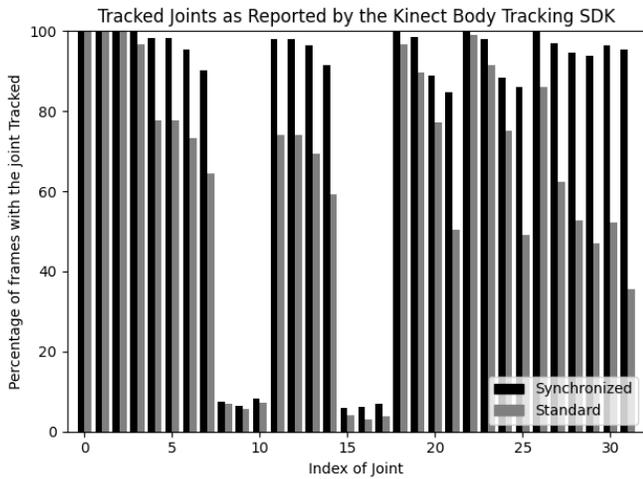
Fig. 8. Percentage of frames in which each joint is tracked. Indices of joints are specified by the body tracking SDK<sup>14</sup>. Small columns: confidence levels for the hand, hand-tip, and thumb.
