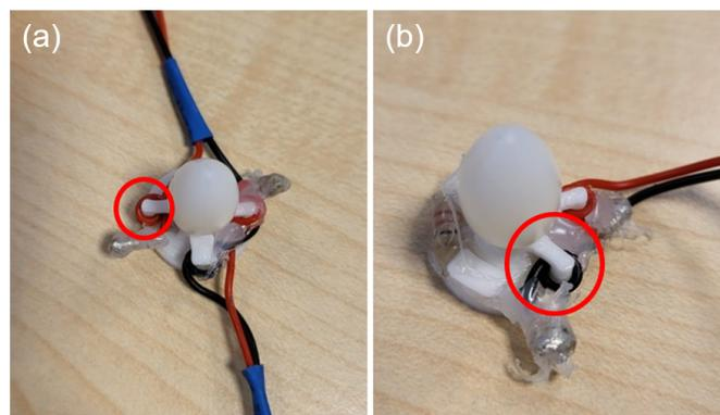
Fig. 2. Two types of marker bases. a) Connecting marker without resistor. b) End marker with resistor. All wires are spun around the strain reliefs (red circles). Soldering is coated with hot glue for isolation and to cover sharp edges.
