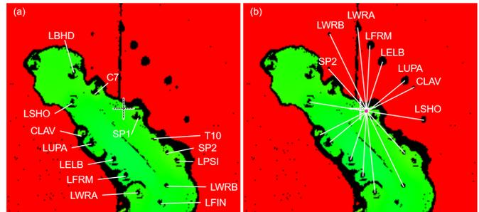
Fig. 5. Cropped depth image of a person doing a squat (side view). Image center is highlighted by a cross. a) Names of markers corresponding to artifacts (SP1 and SP2 are added to spine). b) Markers connected to their corresponding point reflection artifacts. Purple dot: center of reflection.
