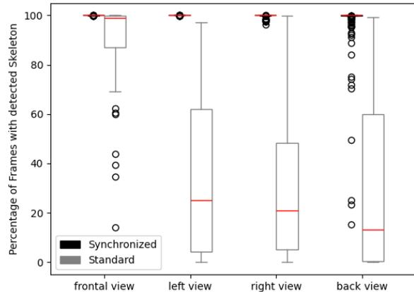
Fig. 7. Percentage of frames where a skeleton could be extracted. Comparison for the front, both sides, and the back between synchronized and standard markers.
